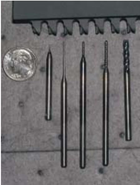
An assortment of diamond-coated tools Keystone Machine uses. Their diameters range from 0.010" to 0.125".
