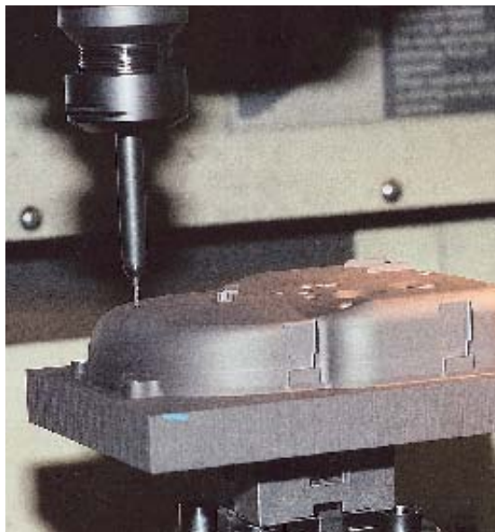
An electrode for producing a plastic mold is milled on a Makino SNC64 machining center at Chicago Mold Engineering.
