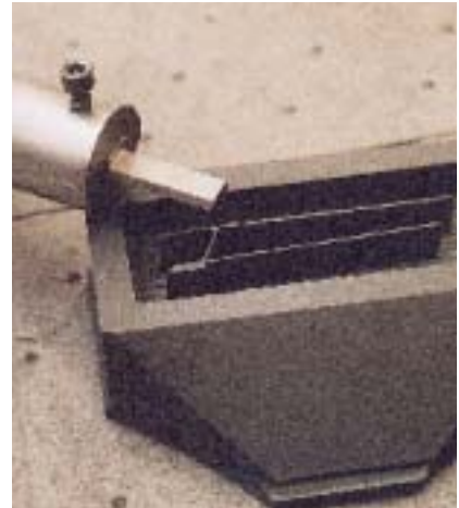
Keystone Tool used this custom broach to machine the internal corners of the graphite electrode it's resting on.
