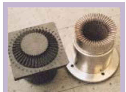
Answer to question on first page: The electrode was used to burn a die that crimps and cuts the paper wrappers that hold Reese's Peanut Butter Cups.
