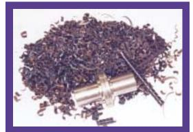
When it comes to optimizing a dry machining process, purple reigns. The chips shown, with their deep purple hue, exemplify a dry machining operation in which a substantial amount of the heat generated by the procedure was transferred away from the tool. The part is an idler shaft for a diesel engine.
