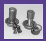
A cold-formed 1035 steel stretch bolt was machined in less than 1 second, with a total cycle time of 3 seconds, using two coated carbide tools under dry machining conditions. The part and the tooling were cool to the touch after the operation. chip control.
