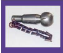
A cold-formed 8640 steel ball stud for a truck steering linkage was machined at 1,800 rpm in less than 1 second using an uncoated carbide tool and cool-to-the-touch dry machining technique. Most of the heat of the operation was carried away by the chips, as evidenced by their deep purple color. Total machining time was 4 seconds. Tool life was 48 hours.
