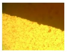
Standard PCD tool edge at 200x magnification. Gaps and nicks in the tool limit the imparted finish to no better than 15µin. to 50µin.
