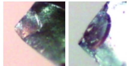
Corners of an endmill run in coolant containing a high level of microscopic particles (60x). The corners have been chipped to the point where they can no longer properly engage the workpiece. When one edge chips, it's likely that the trailing edge will chip, because it slams into the workpiece with more force.
