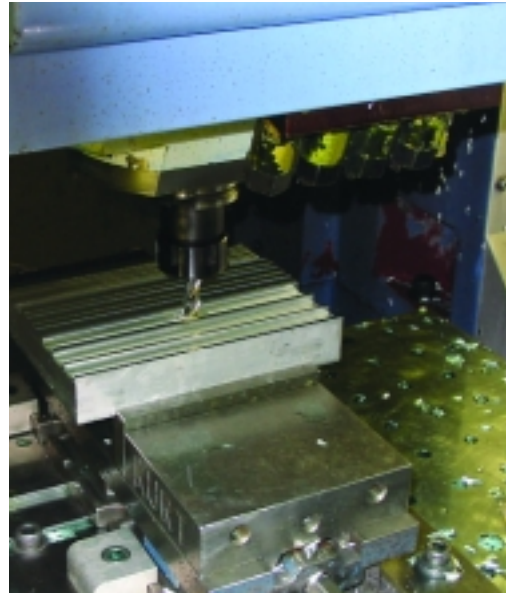
A 3-flute endmill slots a 6061 T-6 aluminum assembly.
