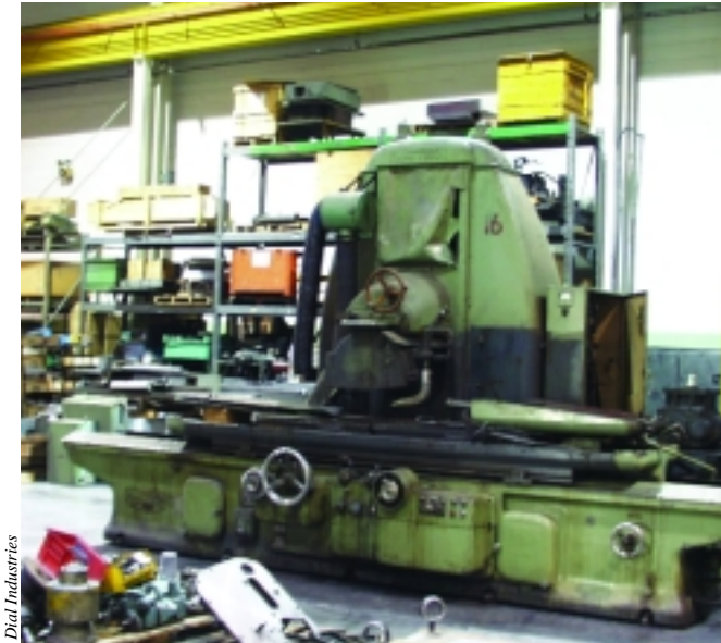
Before-and-after photos of a 45-year-old Mattison grinder that Dial Industries remanufactured.
