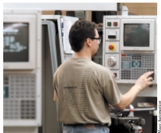
Haas Automation says it designs controls from the operator's and programmer's points of view, with clear function markings and a logically laid-out keypad.
