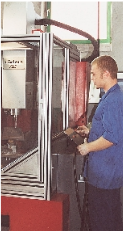
Enclosed high-speed machining centers have reduced complaints about airborne graphite particles.
