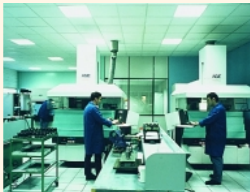
Recent technological advances have made unattended EDMing a reality. Here, operators load programs.
