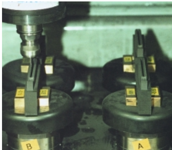
High-speed machining centers facilitate the manufacturing of thin-rib electrodes.
