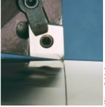
In plunge turning, the entire cutting edge, or a portion of it, is used to make an orthogonal cut (top). That compares to conventional hard turning, in which just the tip of the tool is applied to the workpiece (bottom). deep below the surface before it changes into CRS.
