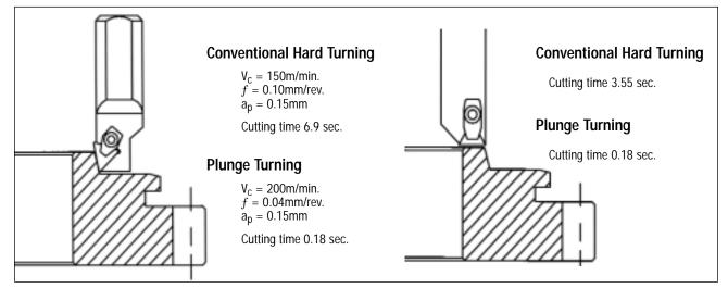
Two examples of the time savings possible when plunge turning a gear compared to conventional hard turning.  $V_c$  = cutting speed, f = feed and  $a_p$  = DOC.
