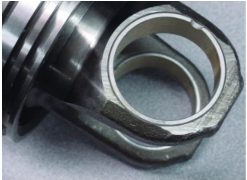
A steelhead piston with a composite bushing pressed into the part's cross-pin bore had to be machined as a single unit to ensure proper clearance between the connecting rod and the piston skirt.
