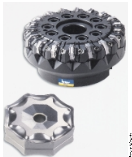
Figure 2: Each of Iscar's octagonal OHNT inserts has 16 cutting edges, an axially positive chip former and a wiper flat.
