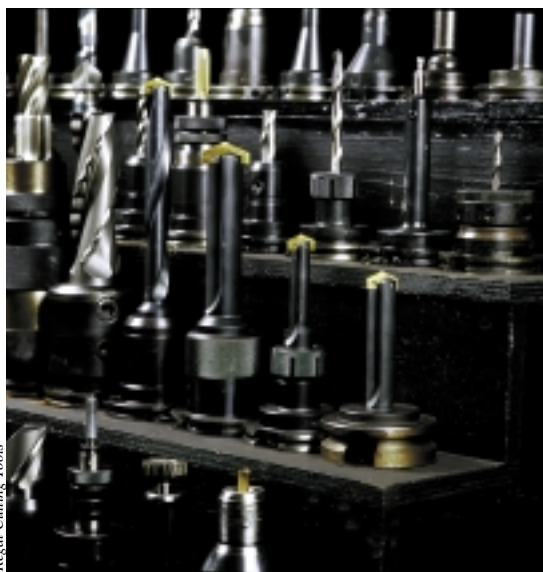
Spade drills are versatile tools for making holes up to 8 diameters deep.
