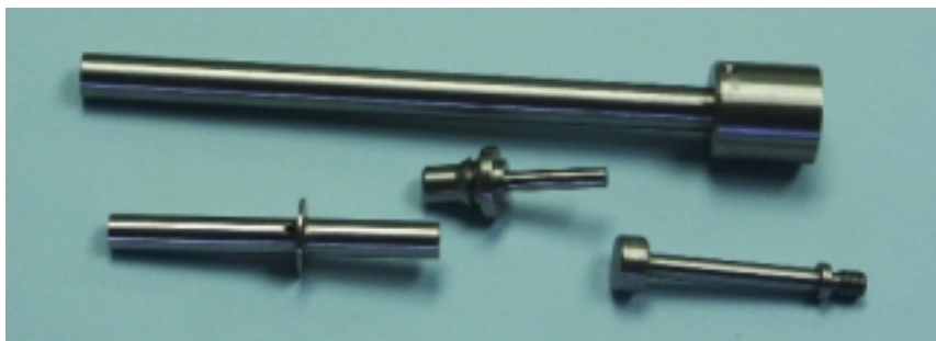
Troublemakers: Parts whose length-to-diameter ratio approaches 3:1 cause machinists all kinds of problems, such as unwanted part tapering and tool chatter.
