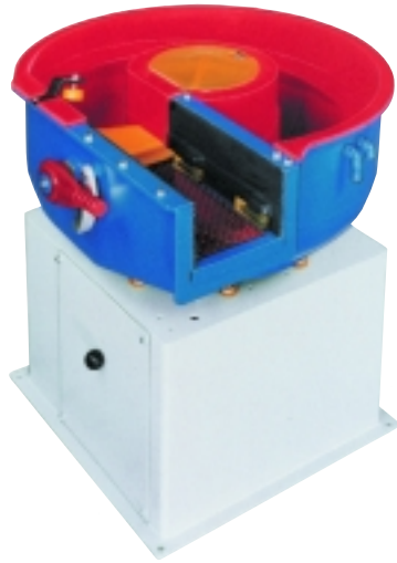
Figure 1: Vibratory bowls—the most popular mass-finishing machines—employ a spiral and oscillating action, causing the finishing media and parts to spiral around the bowl.
