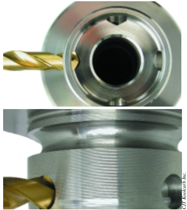
Drilling into convex and irregular surfaces requires a tool with maximum rigidity.
