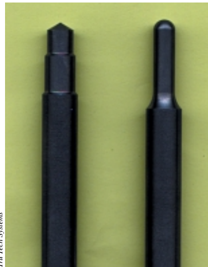
Figure 2: Ground on Tru Tech Systems' 3-axis blank-preparation grinder with a diamond wheel in one setup, the carbide workpiece with two diameters and point (left) was done in 3 minutes and 41 seconds and the blank with radius features took 4 minutes and 32 seconds.
