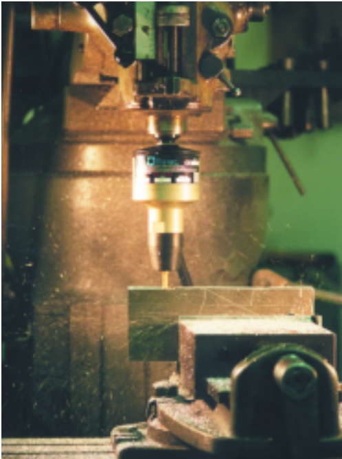
Pneumatic spindles require an unrestricted supply of air to achieve their maximum performance capability.
