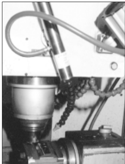
Figure 1: Vortex-type air guns can clear chips from pockets of nearly any depth.
