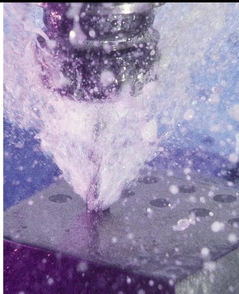
mixed in is to reduce the friction between the tool and workpiece. The rest of the ingredients help the oil stay in emulsion, reduce corrosion and lets users differentiate among brands.
