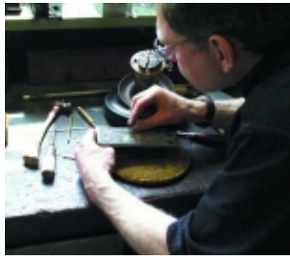
Hand fitting (left) and hand finishing are two of the critical tasks in the manufacture of the Model 37.
