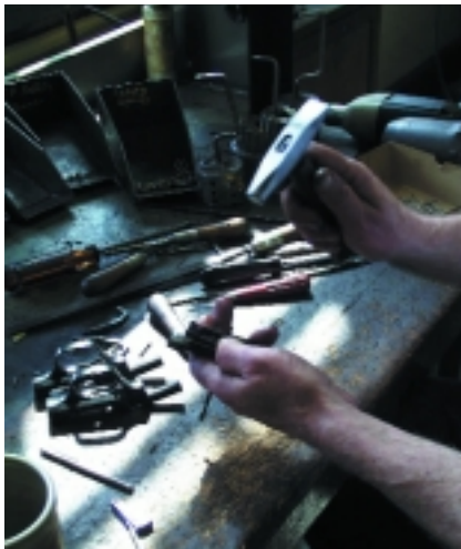
Hand fitting (left) and hand finishing are two of the critical tasks in the manufacture of the Model 37.
