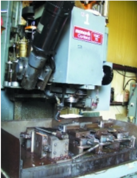
Internal cuts, such as the slide way, are milled on a vertical machining center.
