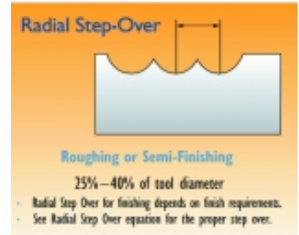
Figure 4: Radial step-over is the distance between centerlines of successive, parallel cuts. A large radial step-over inhibits cooling of the cutter.
