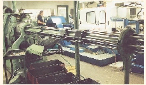
Three rotary transfer machines replaced nine screw machines at Clifton Automatic.
