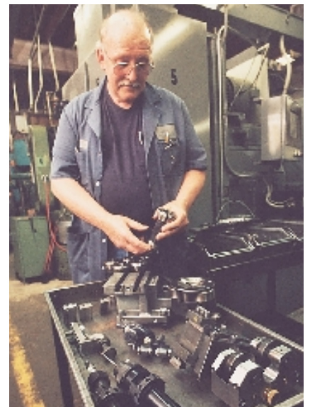
Clifton Automatic’s Jim Hunt preselects tools and toolholders so they can be mounted quickly on a machine.
