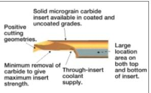
Horn USA's Super-Mini tool is designed for boring holes starting at 0.040" in diameter.
