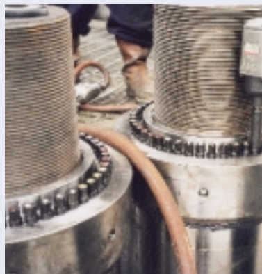
Superbolt thread-mills its mechanical, multiple-jackbolt tensioners, which are available in diameters from 1/2" to 30".
