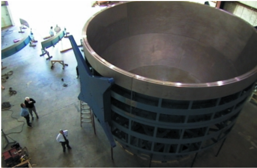
This 25'-high x 27'-dia., dome-shaped mold was produced at Stadco. Machining tolerances were held to 3-millionths of the diameter.
