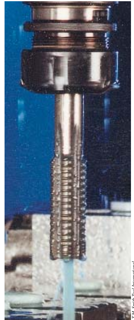
High-pressure through-coolant taps minimize galling.
