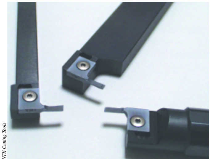
A selection of indexable tooling applicable to most small, Swiss-type CNC lathes.
