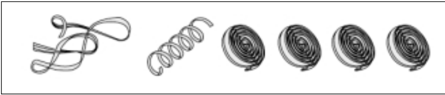
Figure 1: Among the different types of chips are (left to right) long, unformed chips; partially formed “pigtail” chips; and correctly formed “clock-spring” chips.
