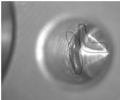
A common deburring-related defect is a burr left in a hole.
