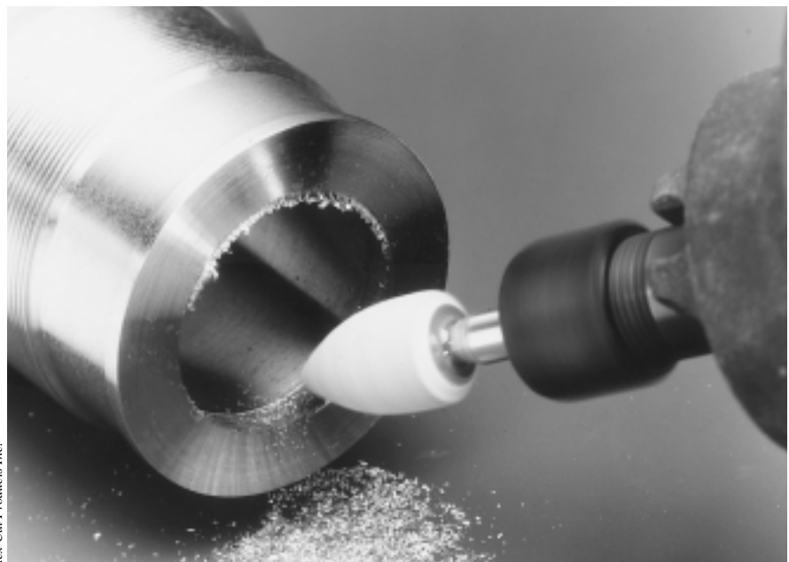
Burrs are undesirable remnants and sharp edges produced by traditional machining processes.
