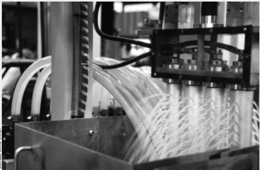
The ECD process is ideal for parts that have hard-to-reach surfaces. This ECD machine is deburring automobile airbag parts.
