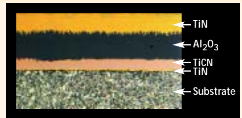
Figure 1: Stellram's Nitro-Lok coating process causes the individual coating layers to interlock, providing a stronger bond than conventional coatings.
