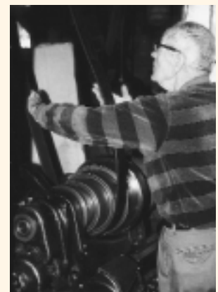
Frank Foriska changes a machine's speed by manually moving the leather belt.
