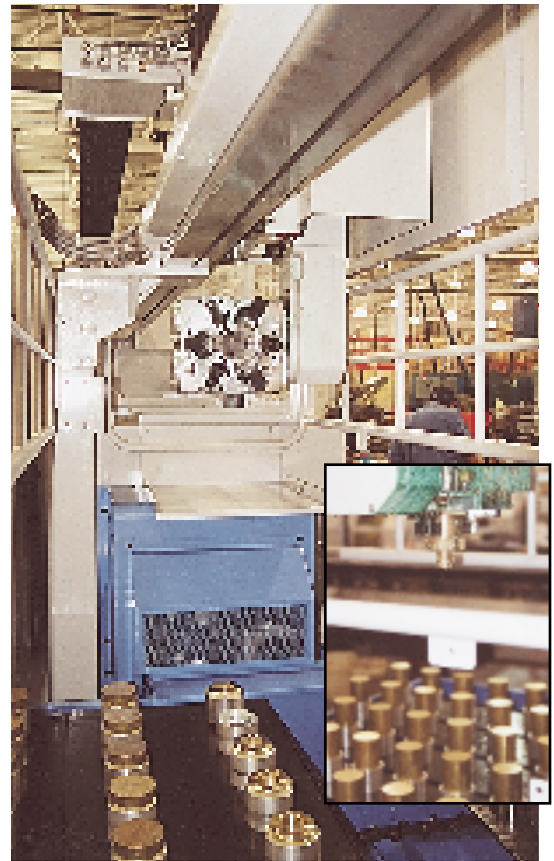
An automated part loader is a popular option. Shown here is a multitask machine and a part being picked up by one of the machine's loaders (insert).
