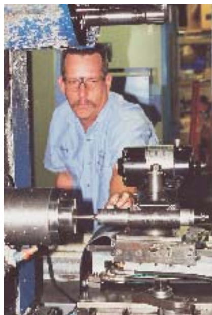
Greg Schurky, a grinding technician for Spindle Grinding Service, regrinds a spindle that was damaged due to a spun toolholder.
