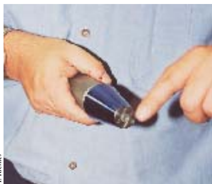
A taper gage is blued-up to determine the bearing surface.
