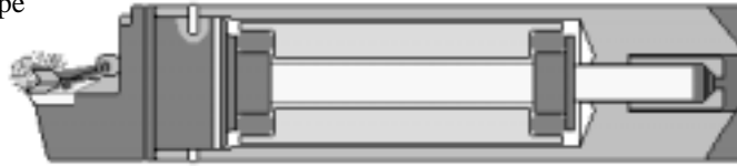
Figure 2: Cross-section of a dampened boring bar.
