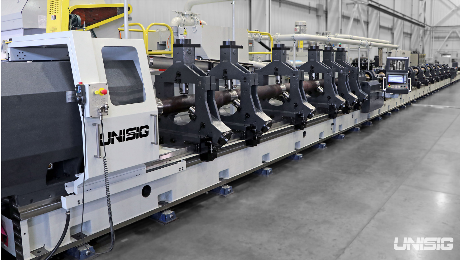
A UNISIG B-Series machine capable of drilling 40 feet [12 meters] deep
