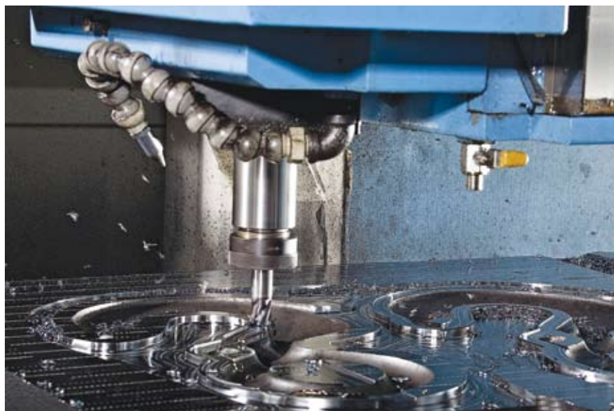
The free-cutting Hi Feed Deka cutter handles 150-ipm feeds when cutting hardened Finkle No. 2 die stock at Crosby-Lebus.
