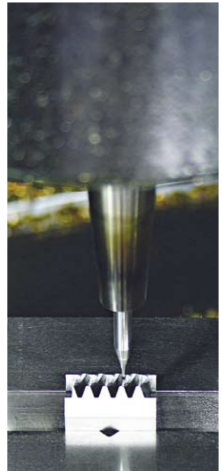
Finish machining of a mold cavity insert with a PCBN microtool.
