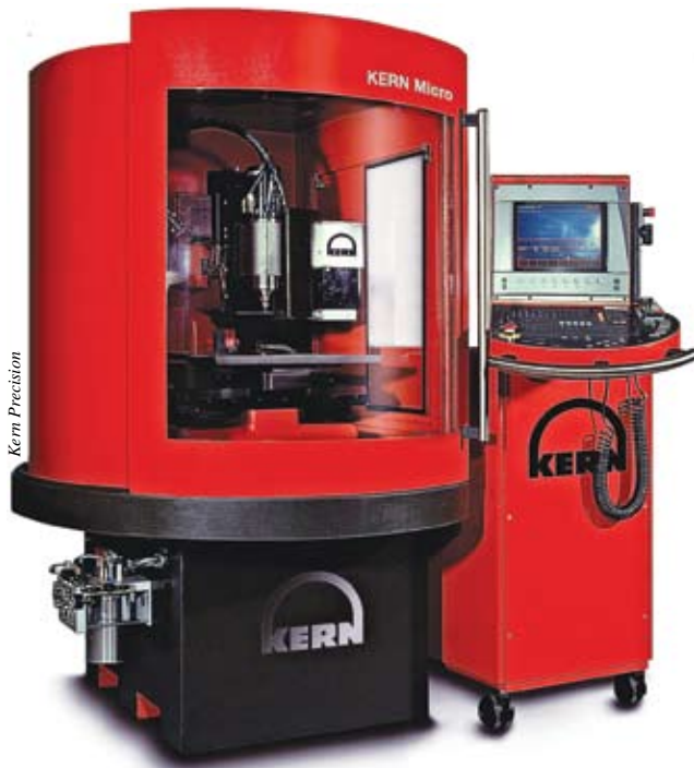
The Kern Micro, which evolved from the company's previous bench-type model, has a footprint of less than 32 sq. ft. and a positioning accuracy of \pm 1\mu\text{m} .
