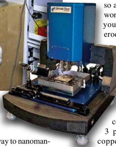
Jerry Mraz, general manager of SmalTec International, with the company's GM703 nanogrinding/microEDM machine. The GM703 has a 10-nanometer step resolution when mechanical micromachining and can generate a spark as small as 0.5µm when EDMing.
