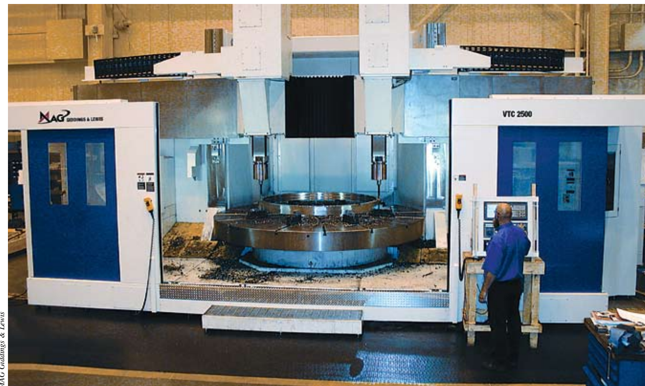
A MAG Giddings & Lewis vertical turning center drilling with two live heads.
