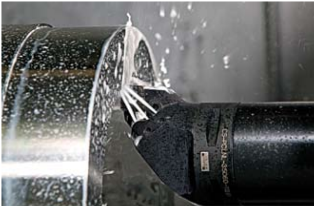
The Sandvik Coromant CoroTurn HP system improves chip control and extends tool life by using high-pressure coolant.
