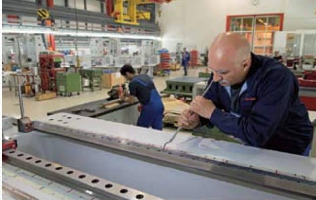
Workers hand scrape ways for a Dixi machine tool.
