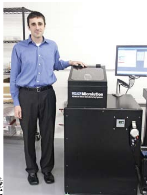
Andy Phillip, Microlution’s president, next to the company’s Model 310-S 3-axis micro milling machine.
