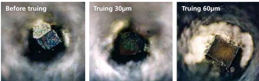
Figure 4: Diamond grains before and after truing to depths of 30µm and 60µm.
