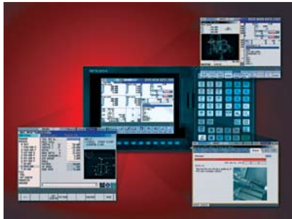
In addition to part-programming assistance (left), CNC screens can provide process-simulation information (upper right) and troubleshooting procedure assistance
