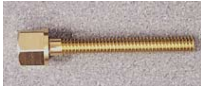
Unfinished part after three segments of turning and threading.
