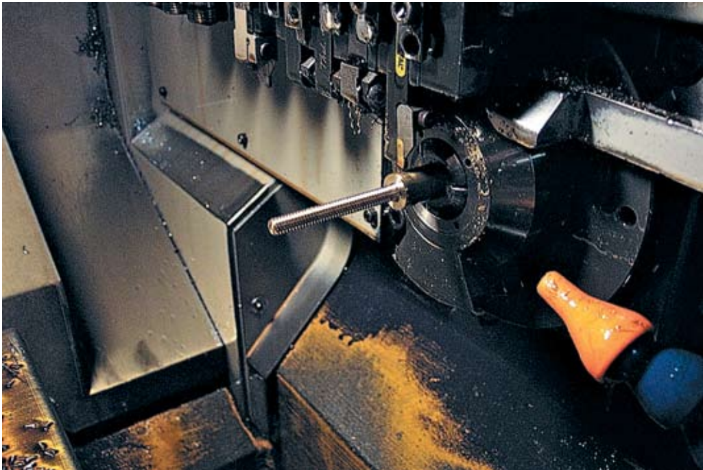
Finished part with 1 \frac{1}{8} " length of \frac{1}{4} -20 threads.
