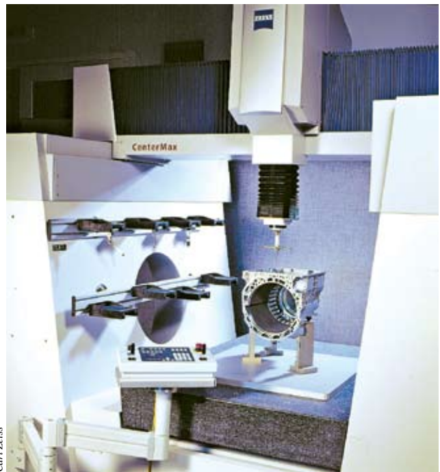
Carl Zeiss' CenterMax CMM is designed to operate as accurately on a shop floor without an enclosure as a CMM in a metrology room.
