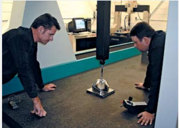
Eric Leene, Redoe Mold Co.'s plant foreman, left, and Chris Tessier, the moldmaker's chief CMM operator, observe as a Wenzel LH 12.30.10 CMM measures a parabolic lens mold.
