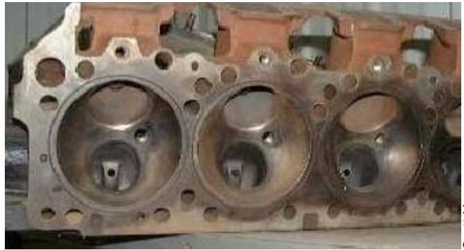
Chrysler’s work in the 1930s on its Xi 220 aircraft engine later benefited its automotive products, such as this 426 Hemi cylinder head.
